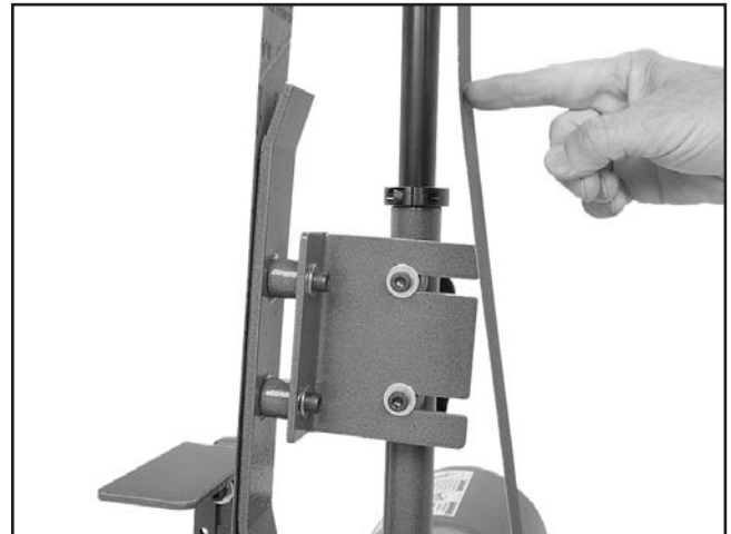
Figure 19. Checking the sanding belt tension.
