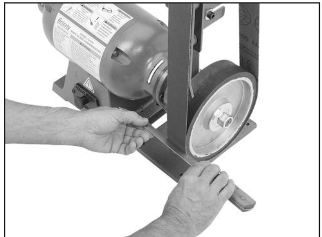
Figure 23. Typical knife grinding operation.
